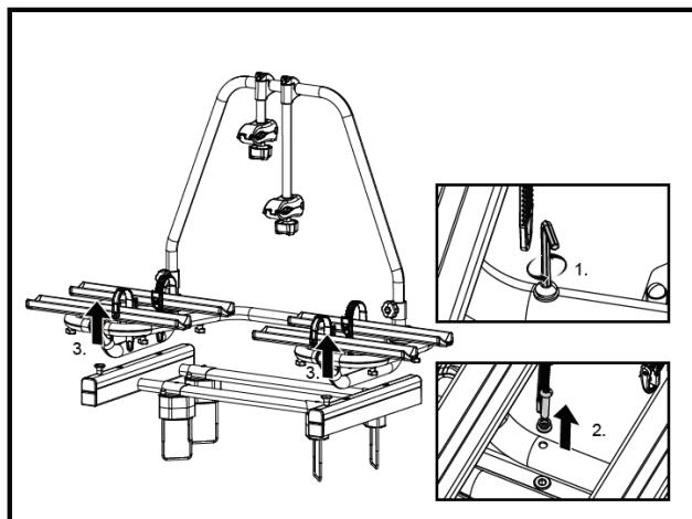
First, loosen the 4 Allen screws (1.) using the Allen key supplied and remove the bolts (2.).
