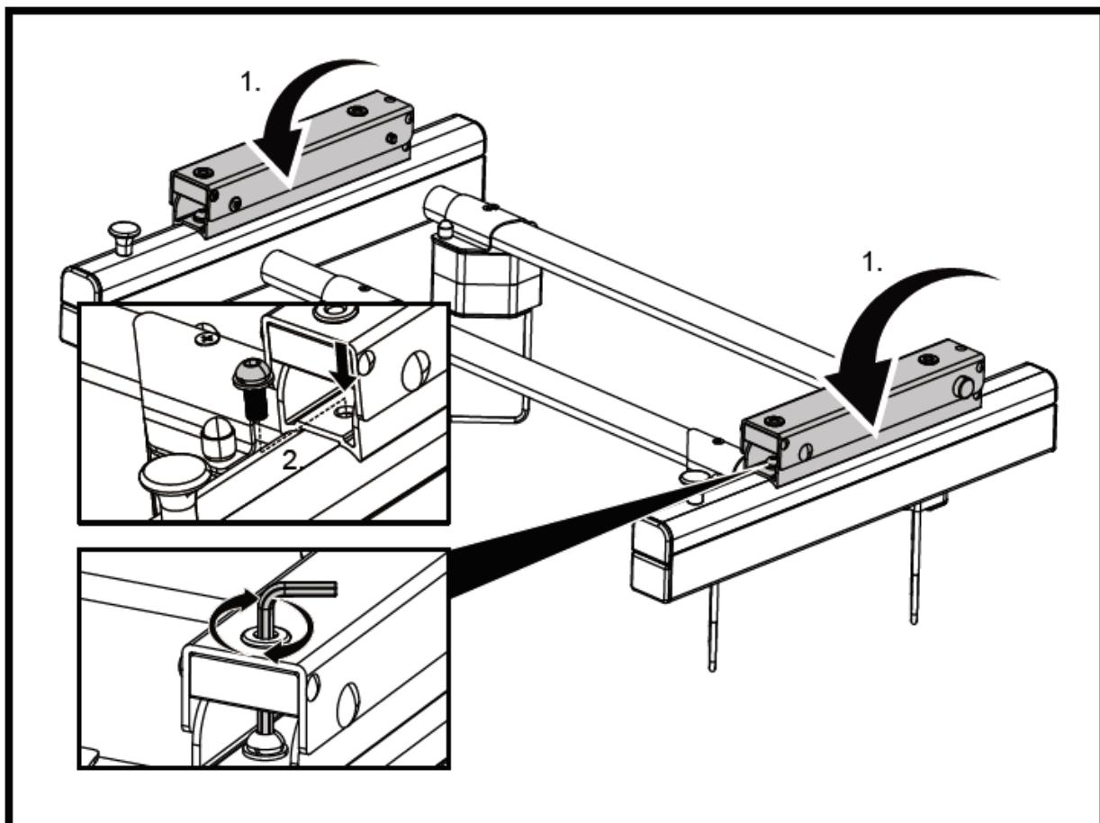
Then mount the rear of the tilting adapters. This is easily done by opening the tilting adapter. To do this, press the button (1.) and open the tilting adapter (2.). Now use the supplied Allen screws M8x25, spring washers M8 and washers M8 and fasten them (3.).
