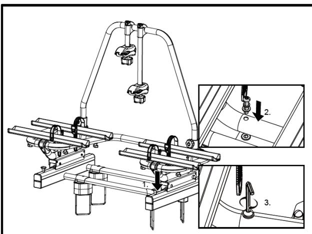
Place the bicycle carrier part on the tilting adapters (1.)
